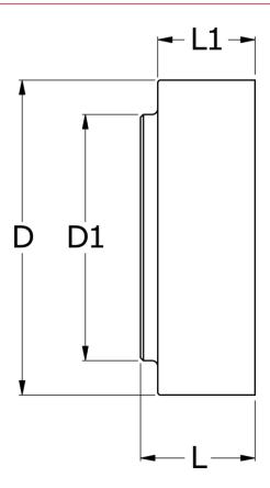
D = 160 D1 = 108 L = 60 L1 = 39 Max bore = 65 Torque (N m) = 560
